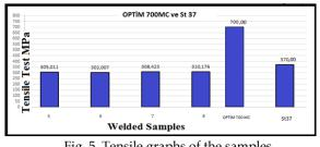
Fig. 5. Tensile graphs of the samples
