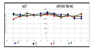
Fig. 7. Microhardness graph of St37- OPTIM 700 MC samples
