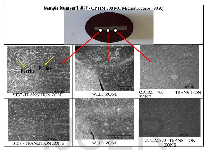
Fig. 3. Sample Number 1 St37 - OPTIM 700 MC microstructure (90 A)
